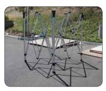
Step 1 Take your frame and slightly expand it open to expose the corner bars.
